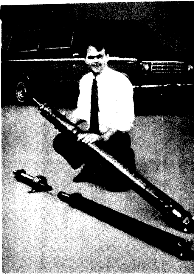
FIGURE 1.19 Filament wound composite power transmission shaft. (Courtesy of Ford Motor Company. Research Staff.)
