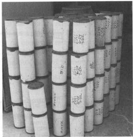
Standard capped cylinders ready for testing.
