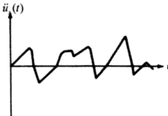
Fig. 5.5 Acceleration function exciting the support of the oscillator in Fig. 5.4.
