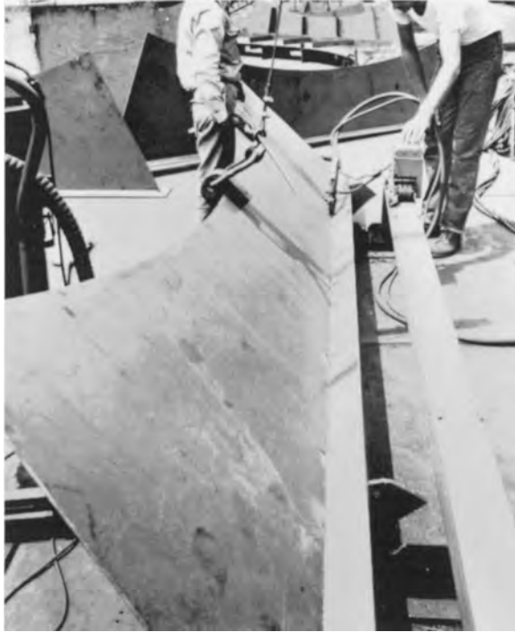
Lincoln ML-3 Squirtwelder mounted on a self-propelled trackless trailer deposits this 1/4-in web-to-flange weld at 28 in/min. (Courtesy of the Lincoln Electric Company.)
